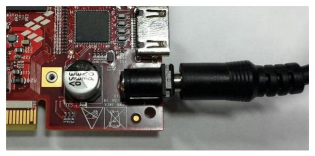
To power-on the board, connect the power supply to J3.
